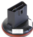
OBDII Volvo/Mack Heavy duty vehicle Connector
