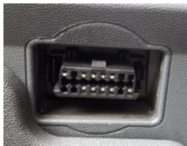
OBDII Volvo/Mack Heavy Duty Vehicle Connector OBDII Light and Medium Duty Vehicles Connector
